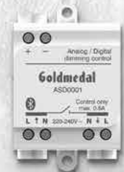
ASD0001 is a BLE-control unit for LED drivers with 0-10V, 1-10V, or DALI dimming interface. The control output can be configured either as analogue 0-10V (and 1-10V) or as a digital standalone DALI control interface.
