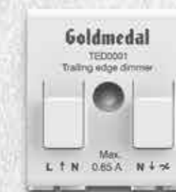
TED0001 is a BLE-enabled trailing-edge dimmer for operation of incandescent lamps, dimmable LED lamps, and dimmable LED control gear. It can be installed in the ceiling, inside a luminaire, or into a ceiling outlet box.
